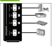
Plug the AV peripheral electronics into the switched outlets.
