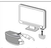
Remove the backing from the double-sided tape on the top of the multi-sensor. Affix the multi-sensor to or near the TV's remote sensor.
