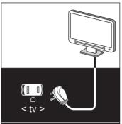
Plug the TV into the control outlet marked <tv>.
